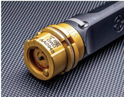
The one of the four radial bolt lugs handle is enough to keep the action safely closed when firing CIP-proof ammunition. The bolt head is complete with a titanium-nitride (TiN) finish.
