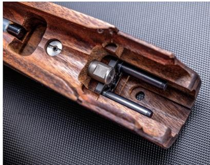
Any tools that are required for changing the barrel or used during disassembly are stowed in the recesses cut within the rifle's forend.
